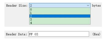
The above figure is taken as an example. The length of frame head is defined as 2, and the content of frame head is defined as FF 03 in hexadecimal:
