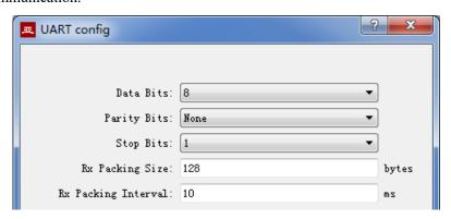
When the UART byte stream is converted into a UDP message or HDLC frame, it is too costly and inefficient if each byte is converted to a UDP message for transmission.
