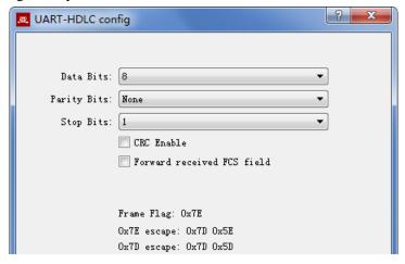
The UART-HDLC frame format adds 0x7E before and after the packet as the opening flag and closing flag with the frame structure is as follows:
