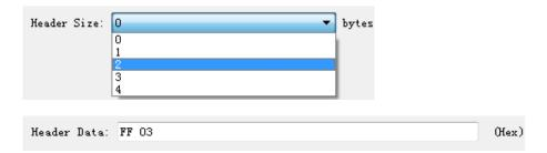
As shown above, the header size is defined as 2, and the header data is defined as FF 03.
