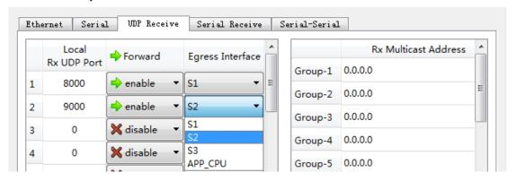
The following configuration realizes the application, where data received from 1 UDP and distributed to 3 serial ports:
