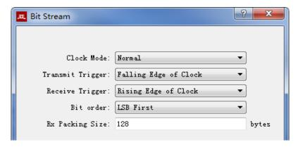
Refer to the HDLC-NRZ parameter configuration for configuration of clock mode, transmit trigger and receive trigger.
