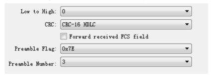
Except for the configuration parameters same as NRZ, parameters with the data line low-tohigh transition definition are included for the Manchester encoding format:
