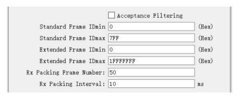
Because the CAN frame is very short, if each CAN frame is converted into a UDP message for transmission, the overhead is too large and the efficiency is too low.
