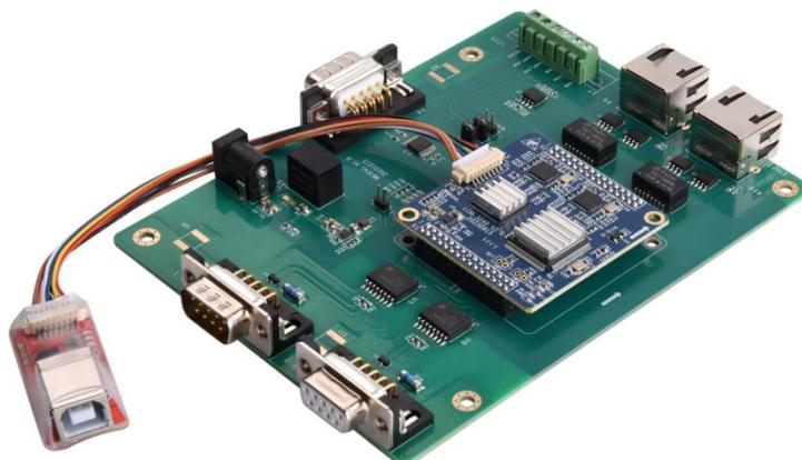
When DMS-UART-8P configuration cable is connected to the management computer USB interface, the computer will add a USB simulation serial port.
